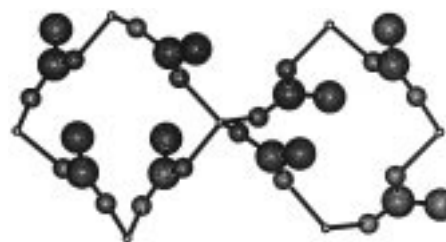
Figure 2. Schematic of proposed structure for dry zinc ethylene–methacrylic ionomers. Same symbols as in Figure 1, except largest filled circles represent carbon. Modeled after diagram appearing in ref 3.
